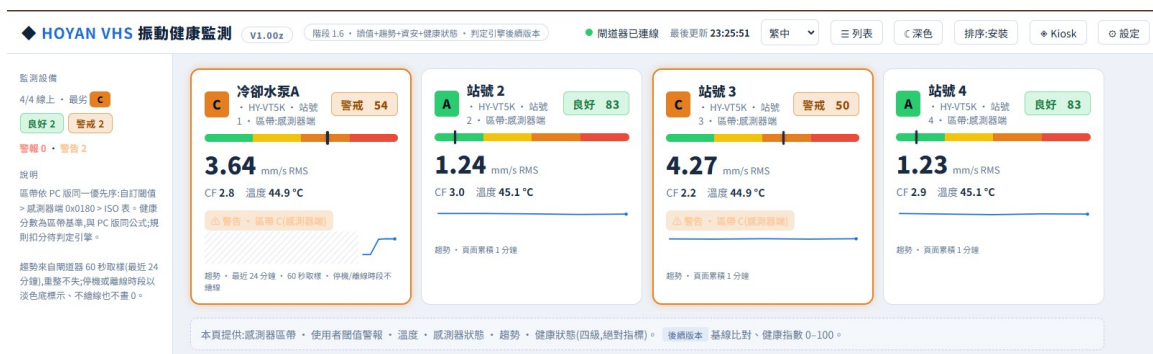
Light theme — two machines in zone C, cards turn to the warning colour
